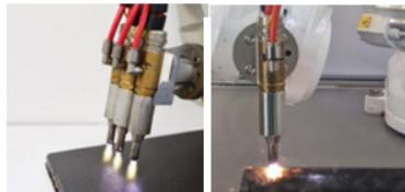
**ULS 3 torch ablation of composite fibre sheet and robotised ablation of composite tube.**
